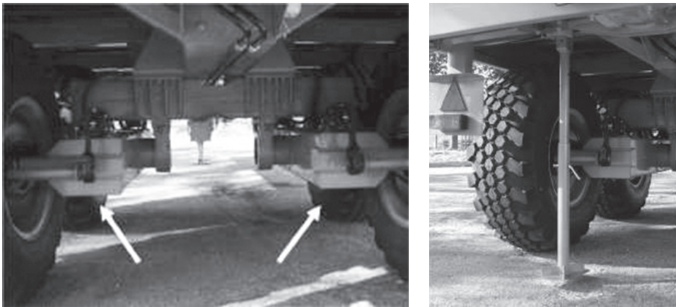
Picture 2. The implemented trailer suspension
